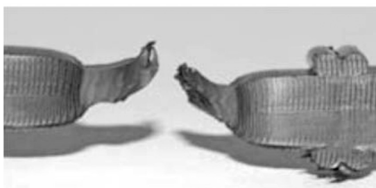
(b) Ductile Rupture Outside Fusion Interface
